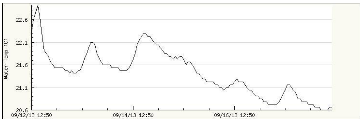
Figure 5. Water temperature at the Sproat fishway from September 12 – September 18, 2013 measured by an HOBO environmental monitoring system.
